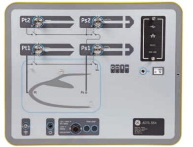
The ADTS554F air data test set is a portable four-channel flightline pitot static tester. In three-channel mode, it provides pitot static air data validation, leak testing, fault-finding and avionics instrumentation testing for any aircraft requiring angle of attack two off static-controlled channels, in addition to a pitot test channel. The ADTS554F can also be used as a standard two-channel flightline air data test set or two simultaneous two-channel air data test sets.
